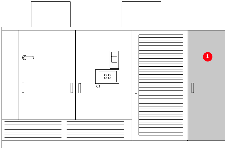
Fig. 26. ACS1000i with (1) braking chopper
